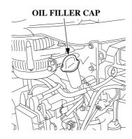
5. Reinstall the oil filler cap securely. Do not overtighten.
