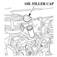
Drain the oil while the engine is still warm to assure rapid and complete draining.
