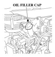
When the engine oil is contaminated or discolored, replace with the fresh engine oil (see page 119 for replacement interval and procedure).
