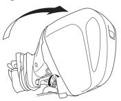
Tilt up the outboard motor using the tilt lock lever when mooring the boat. Shift the control lever into the NEUTRAL position and stop the engine before tilting up the outboard motor.
